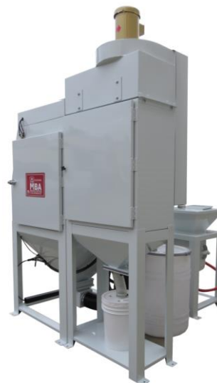
Used Soda Pre-Separator with Pneumatic Conveyor
